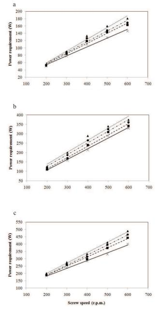
**Fig. 3.** Effect of screw rotational speed and conveying inclination on the power requirements for: a - 15.5, b - 20, and c - 25 cm screw augers; × horizontal conveying,  $\blacksquare 10$ ,  $\bullet 20$ , and  $\blacktriangle 30^{\circ}$ .
