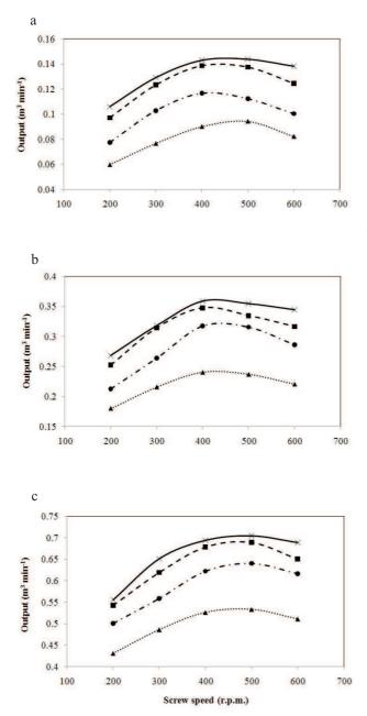
**Fig. 1.** Effect of screw rotational speed and conveying inclination on the volumetric output for: a - 15.5, b - 20, and c - 25 cm screw augers; × horizontal conveying,  $\blacksquare 10$ ,  $\bullet 20$ , and  $\blacktriangle 30^{\circ}$ .
