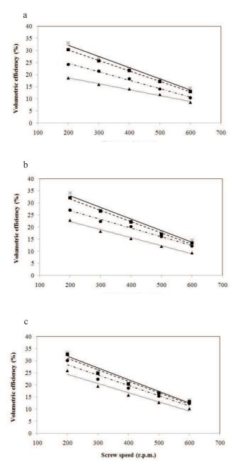
**Fig. 2.** Effect of screw rotational speed and conveying inclination on the volumetric efficiency for: a - 15.5, b - 20, and c - 25 cm screw augers; × horizontal conveying,  $\blacksquare 10$ ,  $\bullet 20$ , and  $\blacktriangle 30^{\circ}$ .
